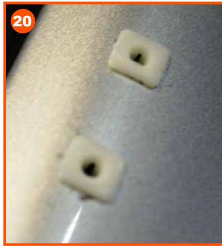
20 Rust proof the holes. Once the rustproof is dry, insert the nylon plugs being careful not to damage the glass
