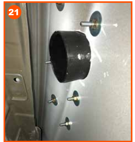
21 Snorkel can now be mounted onto the guard with washers and nuts provided. Tighten mounting bolts evenly.
