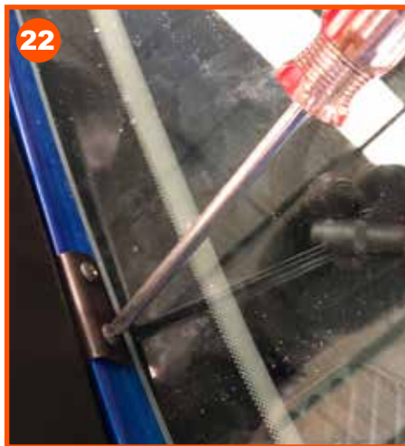
22 Screw the 'A' pillar bracket to the 'A' pillar with button head screws. Be careful not to damage the glass
