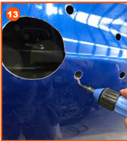
Once happy with the fitment against the guard, remove any burs and rust-proof the holes
