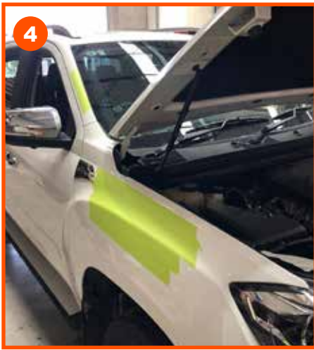
4 Cover work area with masking tape on guard and 'A' pillar
