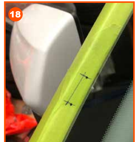
Line up the bracket position with the inner 'A' pillar line to confirm the two holes for the bracket. Centre punch the two 'A' pillar holes
