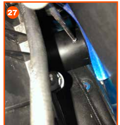
27 Insert a self-taper screw through the top of the air box ducting through the inner snorkel pipe
