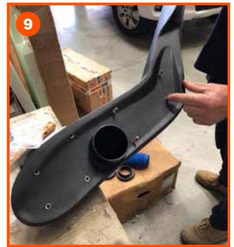
9 Insert studs into the snorkel body (larger stud required for the bottom elbow hole). Do not over tighten
