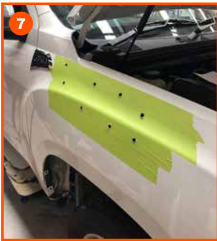
7 Pre-drill all holes with a 3-5mm drill. Drill all mounting holes to 11mm
