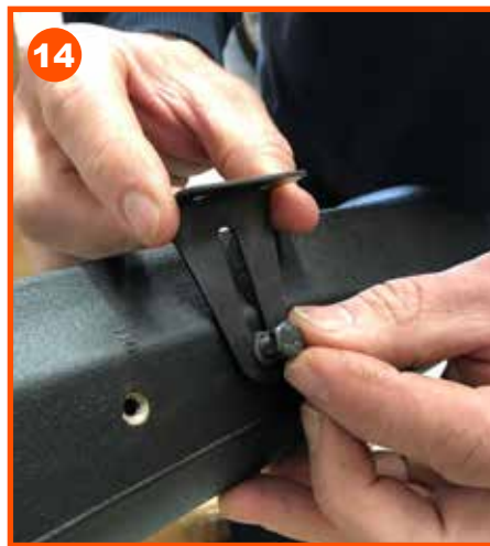
Fit the 'A' pillar bracket to the snorkel loosely, do not tighten.
