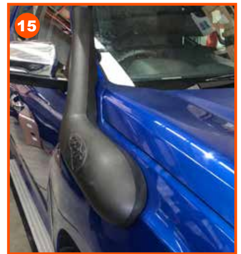
Fit the snorkel on to the guard using only 3-4 nuts
