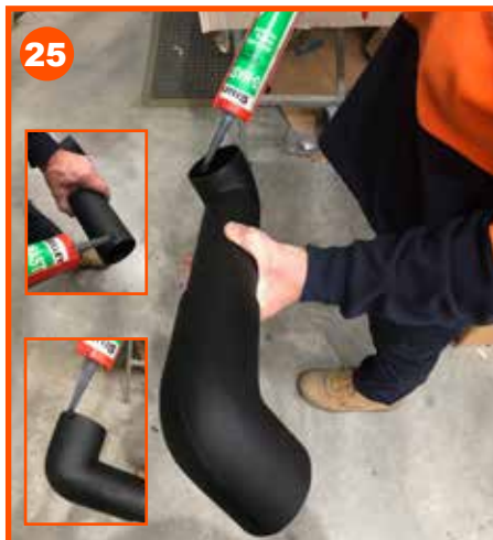
25 Smear sealant inside the join of the inner guard pipe including the section that mounts onto the snorkel and the outside section that mounts inside the air box.
