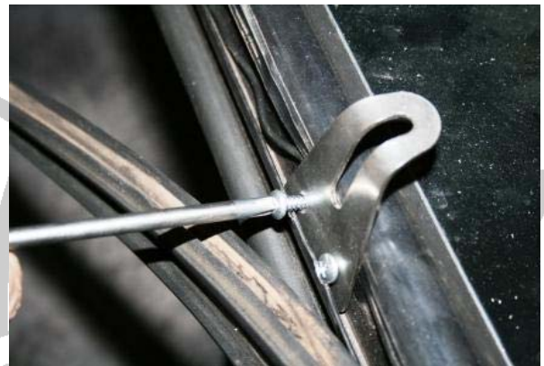
3.57 Secure the "A" Pillar bracket SP043 with the screws SP029
