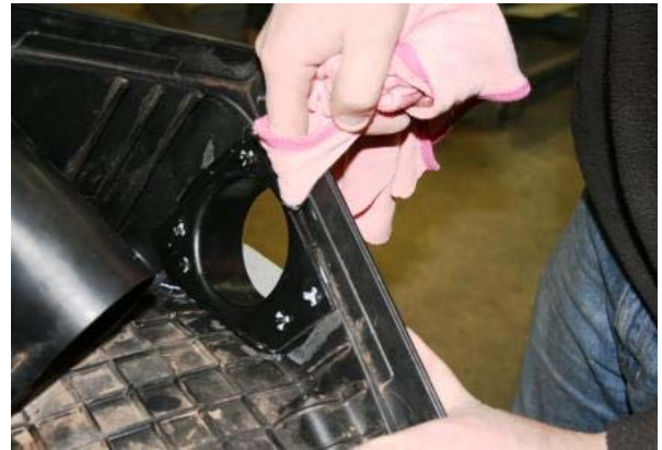
3.27 Remove the excess mastic for a smooth finish
