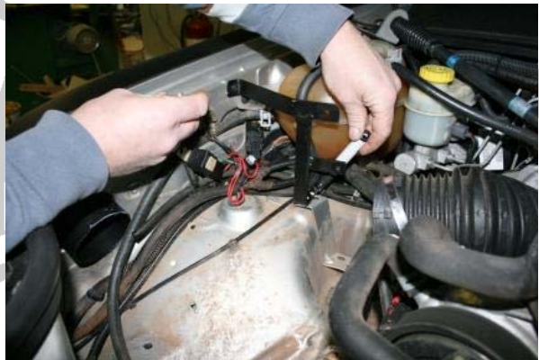
3.63 Secure the relocation bracket SP205 with the top screw retrieved from step 3.8
