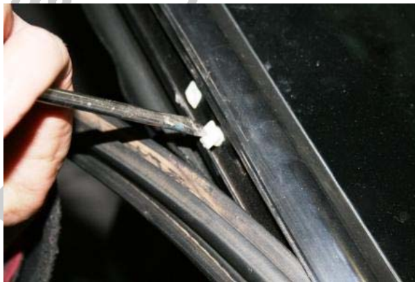
3.56 Fit the two square plugs SP026 (you may need to trim the bottom part of the plugs to allow their insertion)
