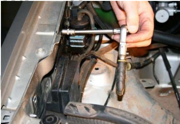
3.7 Unfasten the plenum chamber mounting plate (keep the screws)
