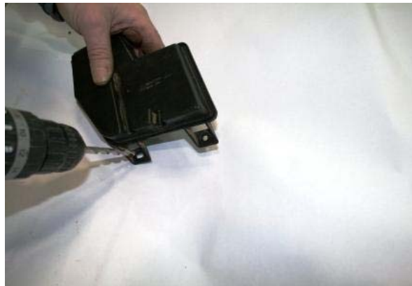
3.12 Increase the size of the two holes to 6.5 mm and elongate the bottom one
