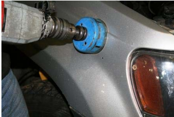
3.41 Using the 90mm hole saw, drill at LOW SPEED the snorkel hole
