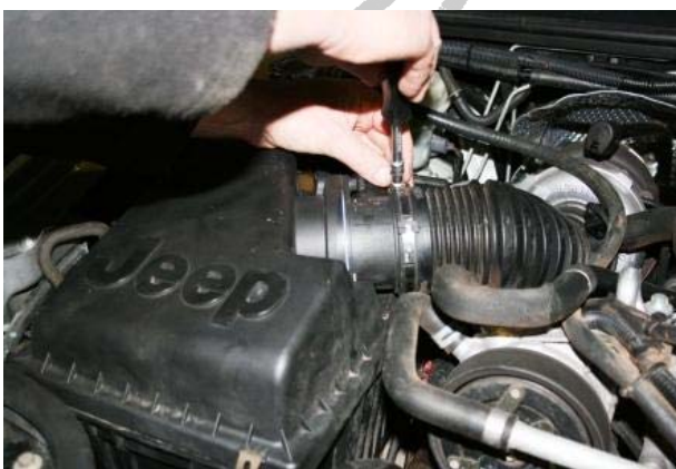
3.81 Re-connect the top hose to the air box and secure the hose clamp
