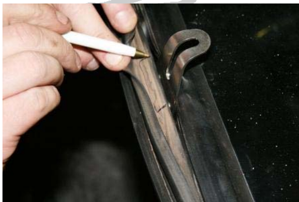
3.58 Refit the rubber seal and mark the location of the bracket on the rubber seal
