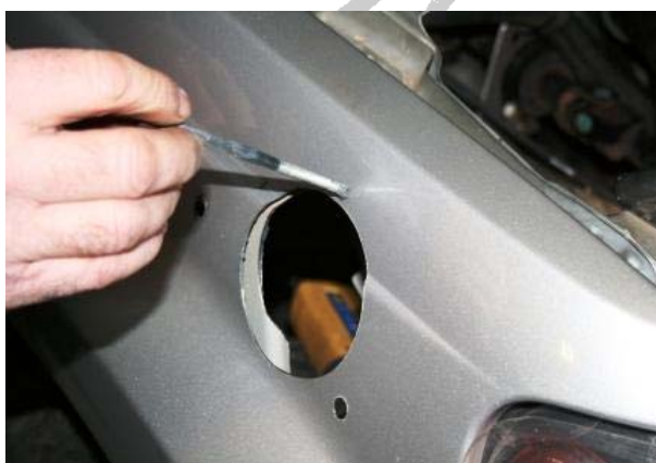
3.45 Paint ALL raw metal surfaces with Zinc rich primer (5 snorkel fixing holes, 1 air intake hole including inside panels)
