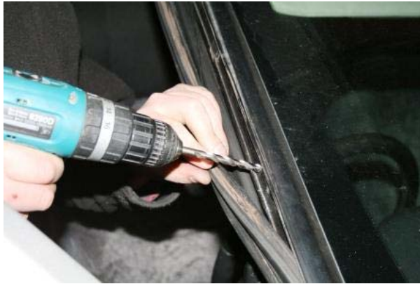
3.54 Using a 7mm bit, drill the two holes for the "A" pillar position
