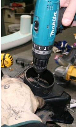
3.19 Using the air box connector SP210 as a template drill a 5mm the pilot hole in the air box
