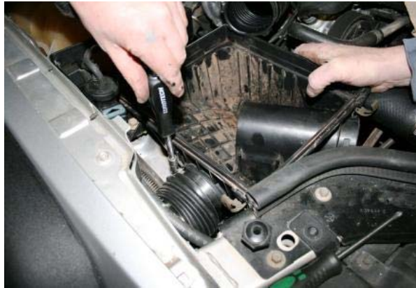
3.78 Tighten the two hose clamps SP018
