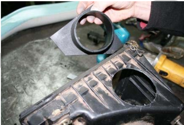
3.21 To ensure proper fitting, place temporarily the SP210 from the inside of the air box.
