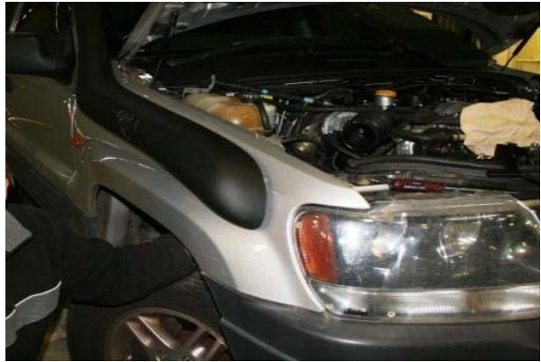
3.61 Secure the snorkel with washers SP025 (x5) and nuts SP027 (x5) to the guard Do not over tighten fixings to avoid damage to the snorkel
