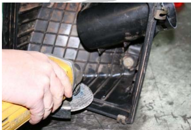
3.17 Grind away the ribs inside the air box...
