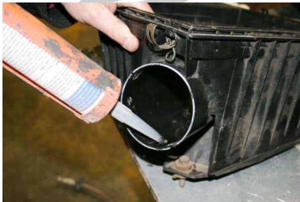
3.30 Apply some mastic inside the air intake
