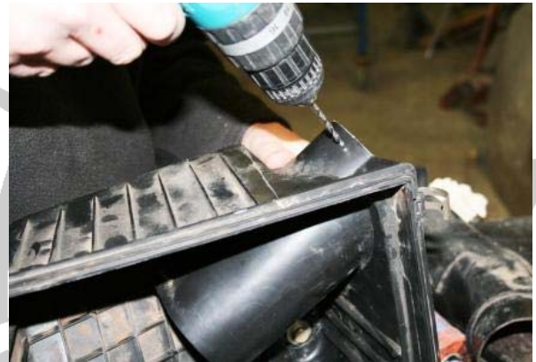
3.29 Using a 4mm bit, drill on three sides, about 120° apart around the air intake and through the SP209
