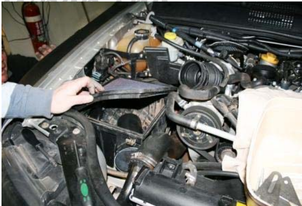
3.79 Re-install the air filter inside the air box
