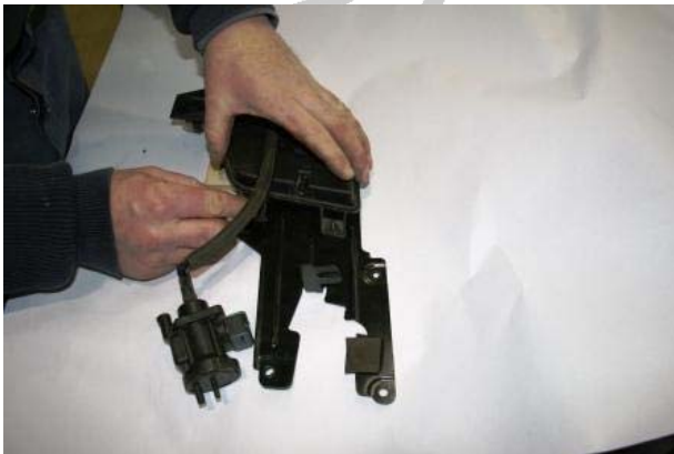
3.9 Remove all the elements from the mounting plate
