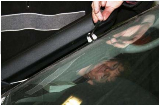
3.62 Secure the snorkel on the "A" pillar bracket with bolt SP024 fitted with spring washer SP023 Do not over tighten fixings to avoid damage to the snorkel
