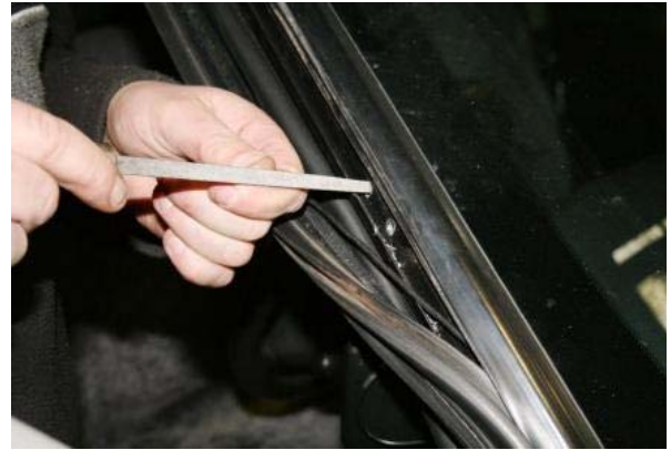
3.55 File the holes with a square file to suit nylon plugs SP026
