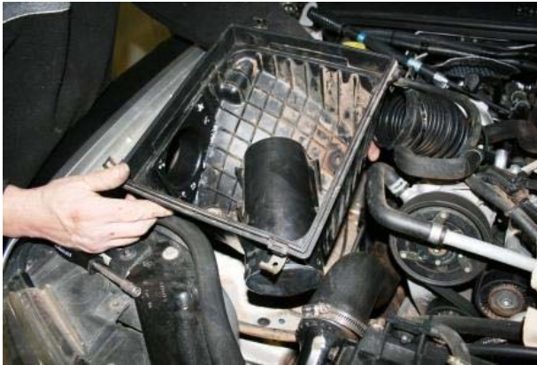
3.77 Re-secure the air box inside the engine bay
