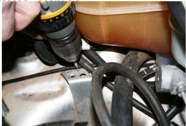
3.67 Using a 5mm bit, drill the location
