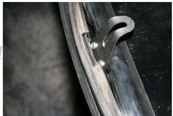
3.59 Using a scalpel, cut the rubber seal along the marks
