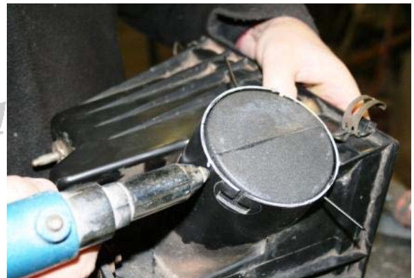
3.31 Insert the air box plug SP209 and rivet it in place
