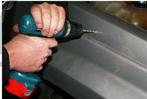
3.37 Using a 5mm bit, pre-drill all holes (5 snorkel mounting holes, 1 hole saw hole)
