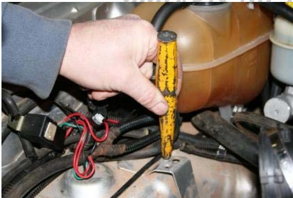
3.65 Remove the bracket SP205 3.66 Punch the location
