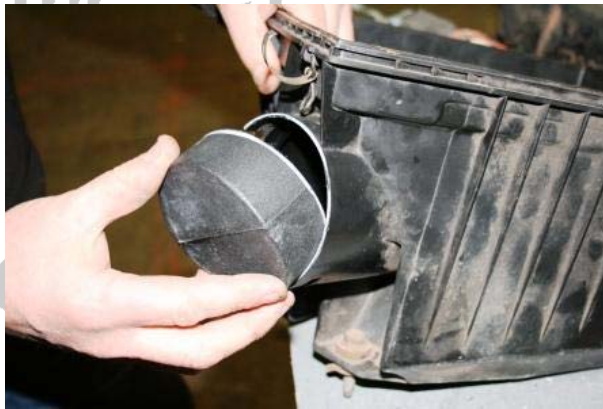
3.28 Insert the air box plug SP209 flush in the unused air intake
