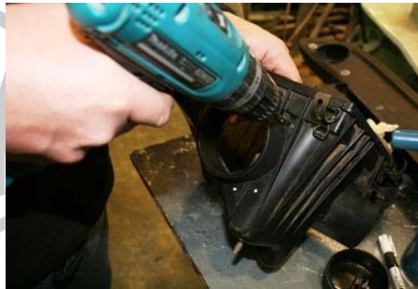
3.23 Using a 4mm bit, drill 4 holes through the air box and the SP210
