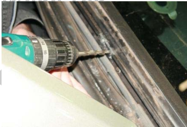
3.59 Using a 7mm bit, drill the two holes for the "A" pillar position
