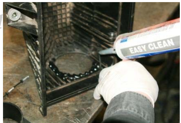
3.19 Remove the SP210 3.20 Fill the voids between the ribs with mastic
