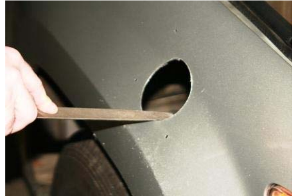
3.44 File the edge of the hole to remove any bur
