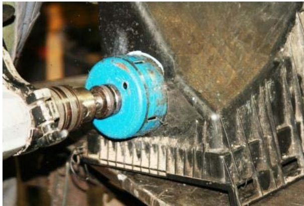
3.13 Using the 90mm hole saw, drill at SLOW speed a 90mm hole in the air box
