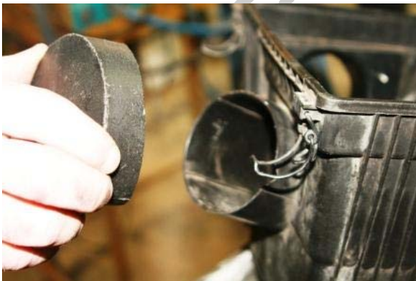
3.25 Insert the air box plug SP212 over the unused air intake ensuring it completely covers the slots
