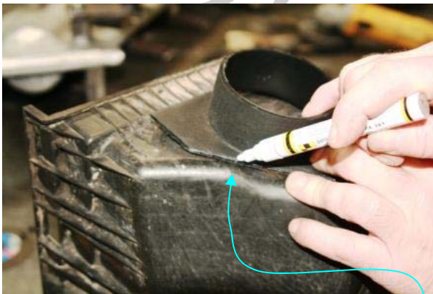
3.10 Using the air box connector SP210 as a template, mark the location to be drilled
