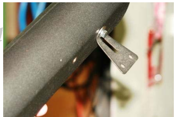
3.48 Fit the "A" pillar bracket SP043 with the washer SP023 and bolt SP024 Do not over tighten fixings to avoid damage to the snorkel
