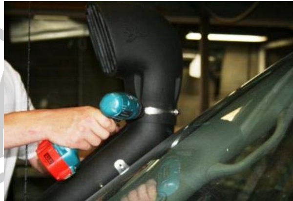
3.84 Drill the hose clamp next to the worm drive
