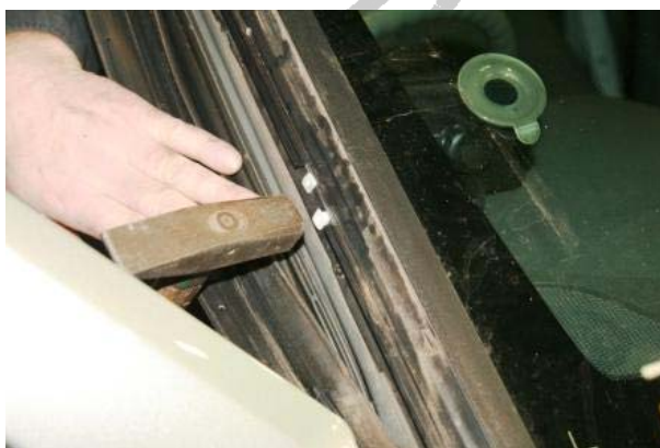
3.61 Fit the two square plugs SP026
