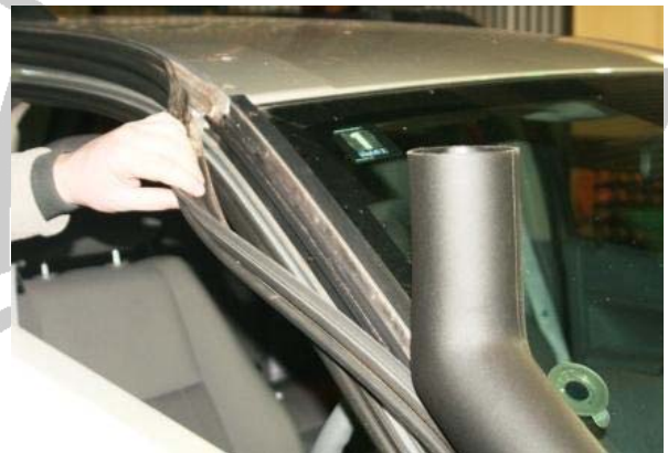
3.76 Refit the rubber seal in place
