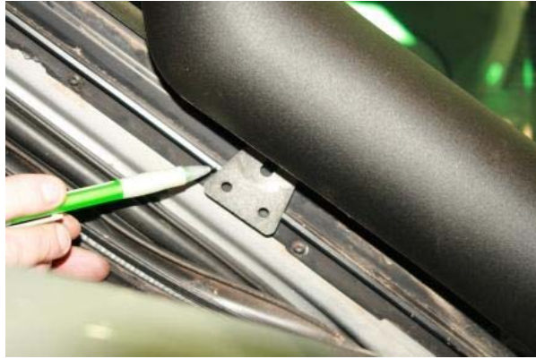
3.50 Mark the edges of the "A" pillar bracket onto the plastic lining
