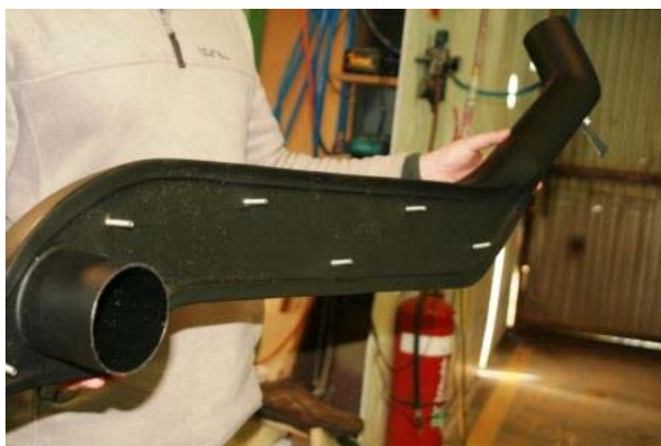
3.47 Fit the seven studs SP022 (20mm must protrude) and secure them with a locking compound
