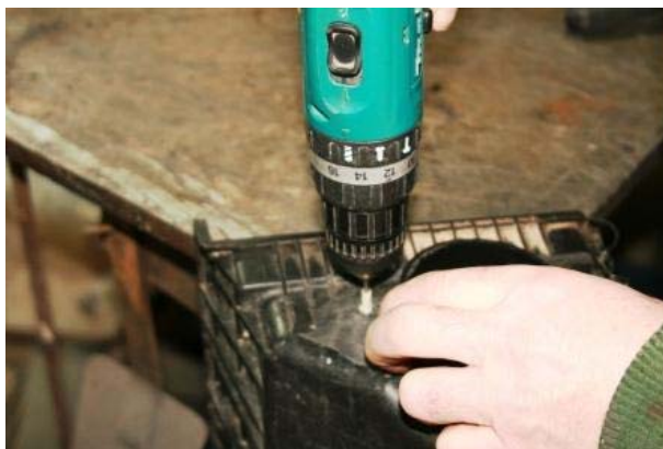
3.18 Using a 4mm bit, drill 4 holes through the air box and the SP210
