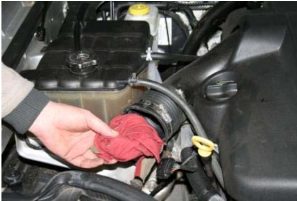
3.5 Protect the air intake by placing a rag inside
