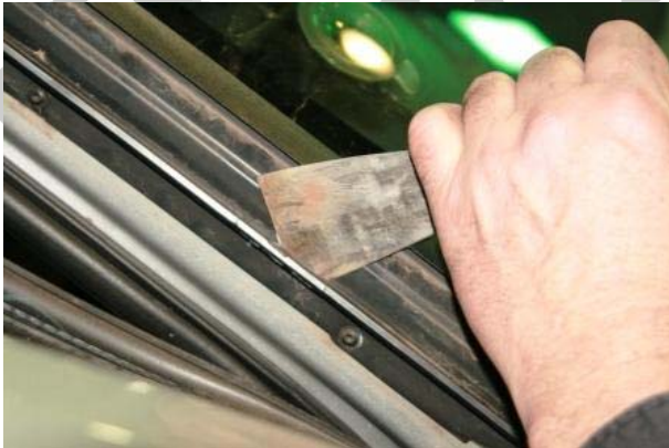
3.52 Using a sharp chisel, cut the excess material...
