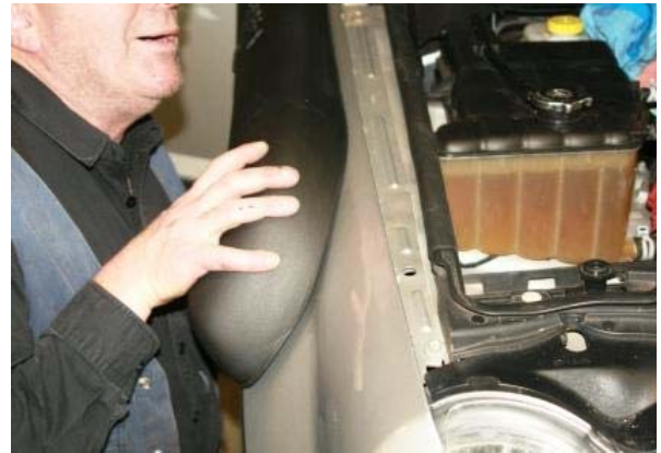
3.74 Secure the snorkel with washers SP025 (x7) and nuts SP027 (x7) to the guard Do not over tighten fixings to avoid damage to the snorkel
