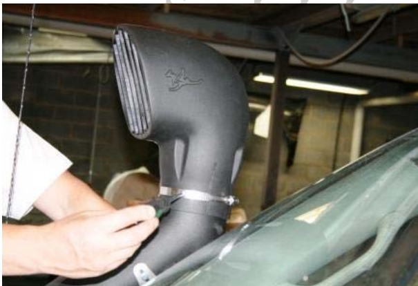
3.85 Secure the Air Ram with the self tapping screw SP029
