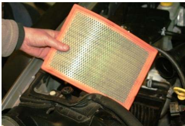
3.77 Re-install the air filter inside the air box
