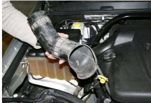
3.6 Remove the air intake and discard it
