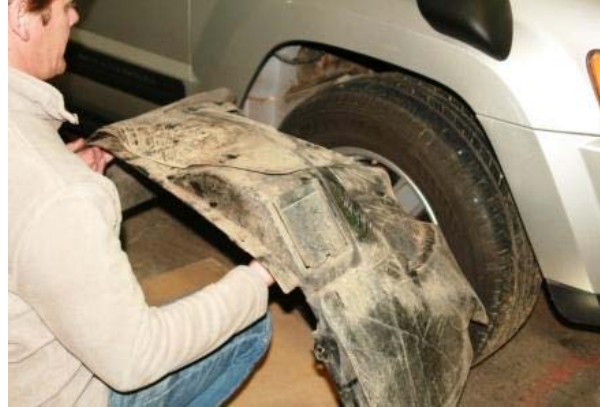
3.81 Refit the splash guard
