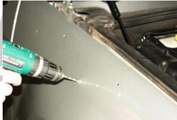
3.39 Using a 5mm bit, pre-drill all holes (7 snorkel mounting holes, 1 hole saw hole)
