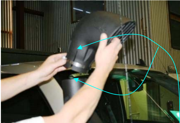
3.82 Slide the hose clamp SP018 on the air ram SP063 then slide it on the snorkel SP196
