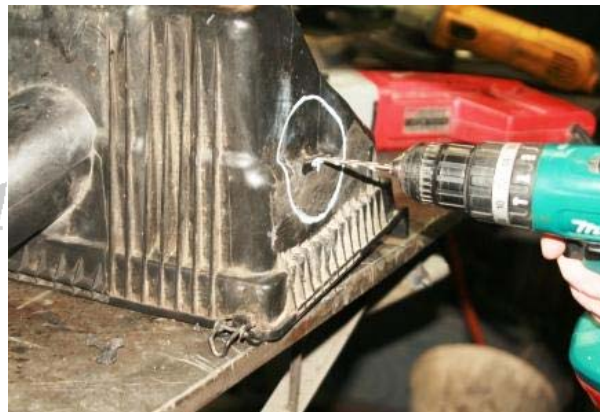
3.12 Drill a 5mm the pilot hole in the air box
