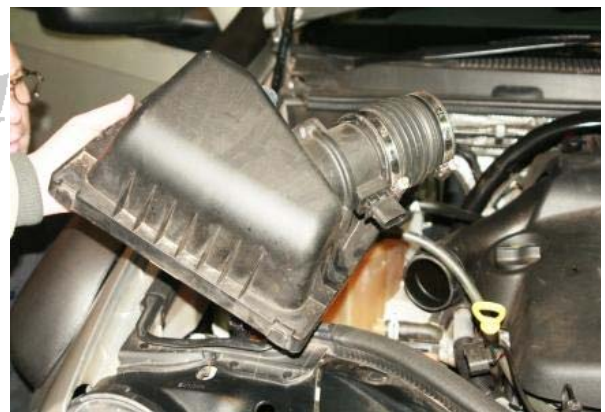
3.78 Close the air box 3.79 Remove the protection rag
