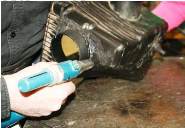
3.23 Secure it with four pop rivets
