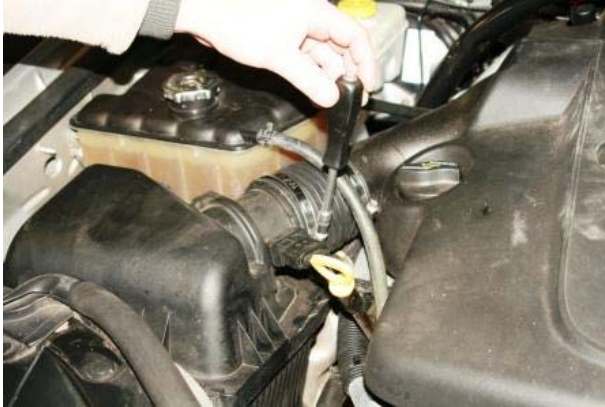
3.80 Re-connect the top hose to the air box and secure the hose clamp
