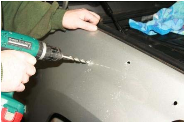
3.40 Cover with masking tape 3.41 Using a 10mm bit, drill the 7 fixation holes (not the snorkel hole)
