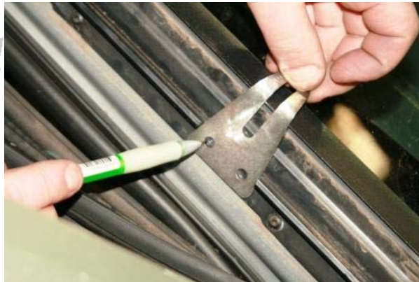
3.56 Place the "A" pillar bracket SP043 in the slot and mark the location of the two holes
