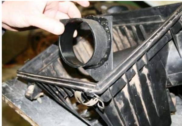
3.22 Re-install it inside the air box
