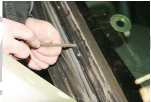
3.60 File the holes with a square file to suit nylon plugs SP026
