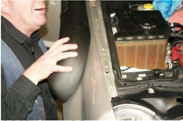
3.49 Pre fit the snorkel to the guard to allow the marking of the "A" pillar bracket
