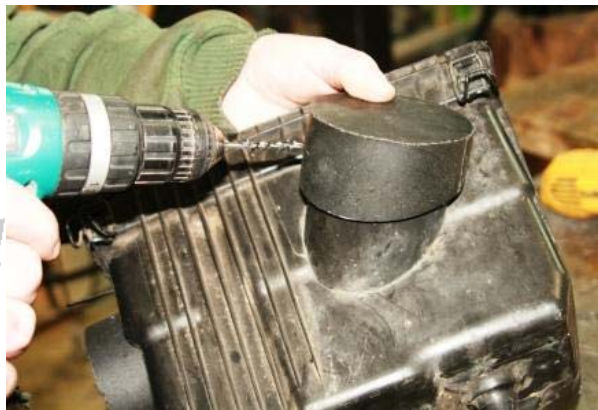
3.26 Using a 4mm bit, drill on three sides, about 120° apart, around the air box plug SP212 and through the air intake
