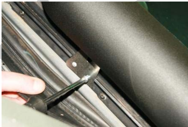
3.75 Using the two self tapping screws SP029, secure the "A" pillar bracket
