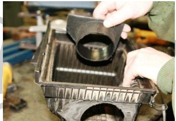
3.16 To ensure proper fitting, place temporarily the SP210 from the inside of the air box.
