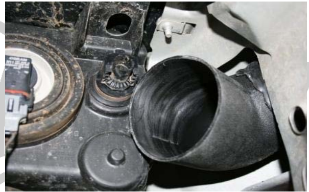
3.68 Slide back the TPR hose backward until only the SP137 protrude in the engine bay
