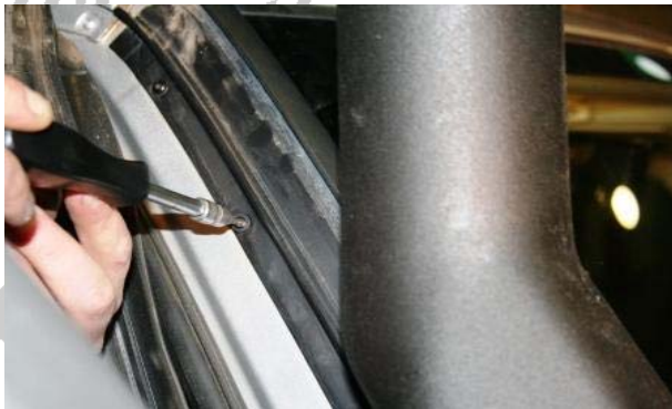
3.41 Refit the black strip on the "A" Pillar
