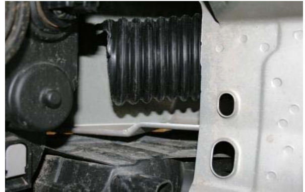
3.64 Slide the TPR hose through the inner guard inside the engine bay
