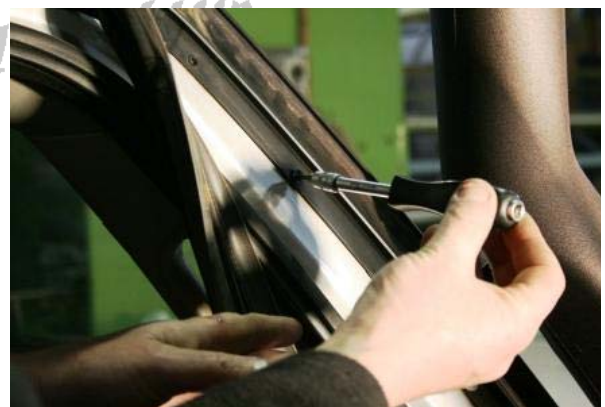
3.38 Remove the black strip from the "A" Pillar
