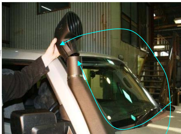
3.78 Slide the air ram SP063 onto the snorkel
