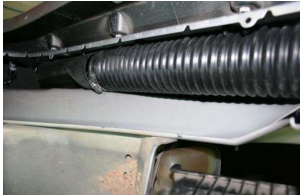
3.73 Connect the other side of the TPR hose to the SP165
