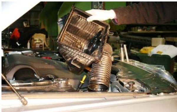
3.69 Slide back the air box base assembly in the engine bay
