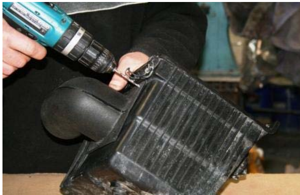
3.14 Use the connector as a template to drill seven 4mm holes in the air box
