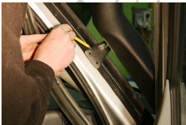
3.37 Mark the "A" pillar bracket position on the black strip
