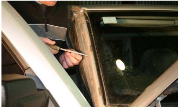
3.47 File the holes with a square file to suit nylon plugs SP026
