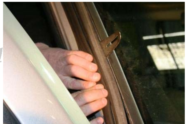
3.52 Re-fit the rubber seal onto the A Pillar
