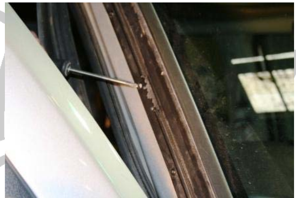
3.50 Refit the black strip but omit the screw next to the bracket
