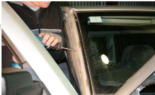
3.46 Then drill the two holes at 7mm
