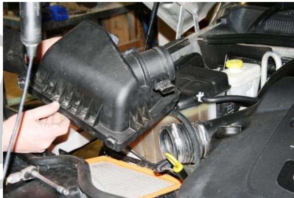
3.76 Refit the cover of the air box and reconnect the outlet tube and sensing cables
