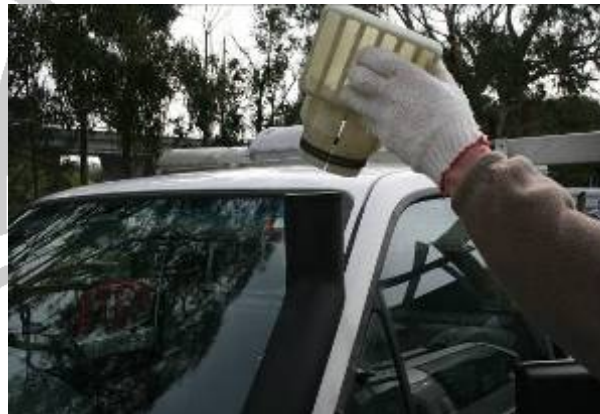
4.4 Re-install the Air ram SP063
