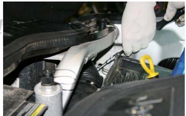
3.70 Connect the TPR hose to the elbow SP137
