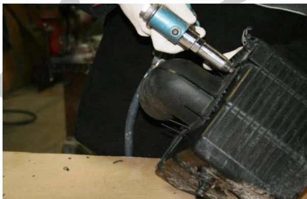
3.18 Using the rivets SP112, attach the SP175A to the air box
