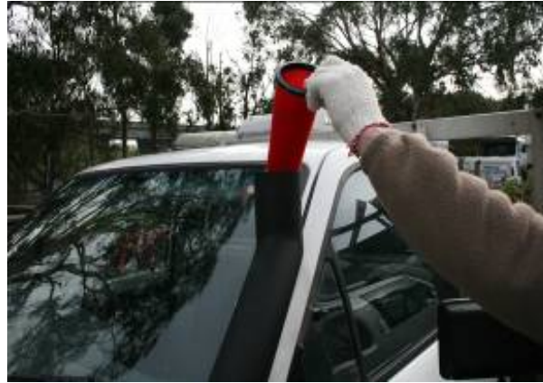
4.2 Install Pre-cleaner filter sock SP065B
