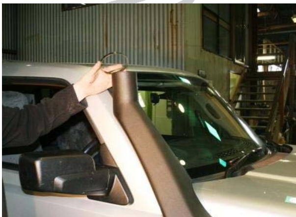
3.77 Slide the hose clamp SP018 on the snorkel SP168
