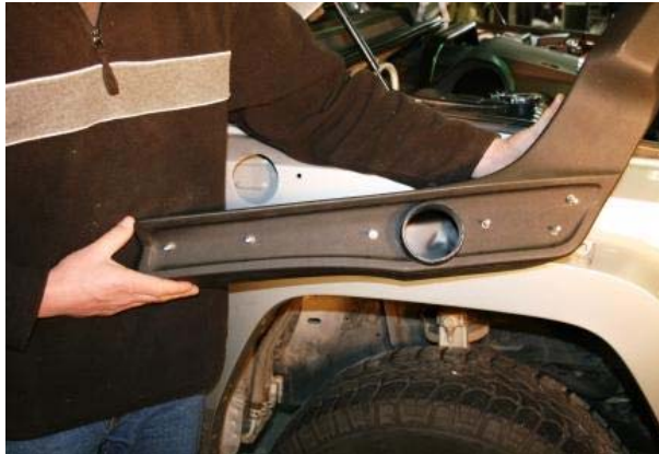
3.33 Screw the 6 studs SP022 with chemical locking compound; at least 20mm must protrude
