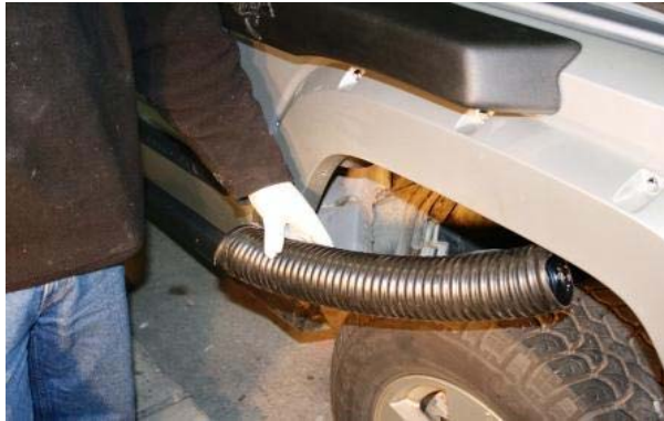
3.63 Position the TPR hose SP015 this way under the guard, ensuring that the hose clamp faces the back of the car
