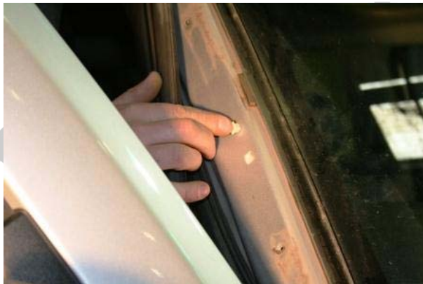
3.49 Once the paint is dry, fit the 2 square plugs SP026
