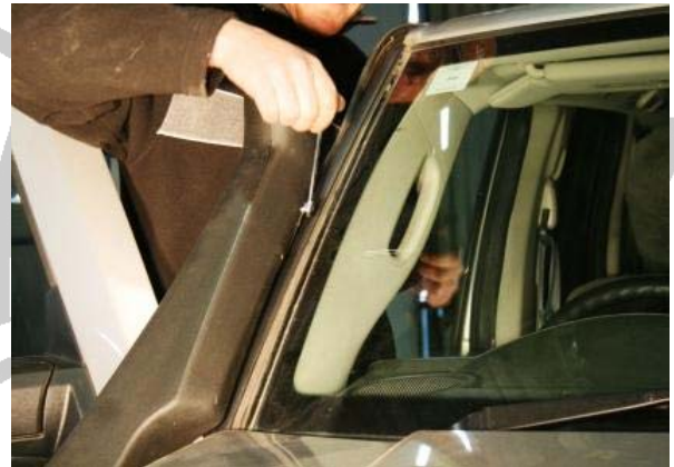
3.36 Fit the "A" pillar bracket SP174 with the washer SP023 and bolt SP024 Do not over tighten fixings to avoid damage to the snorkel
