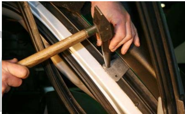
3.42 Place the "A" Pillar bracket in the slot and centre punch the 2 holes
