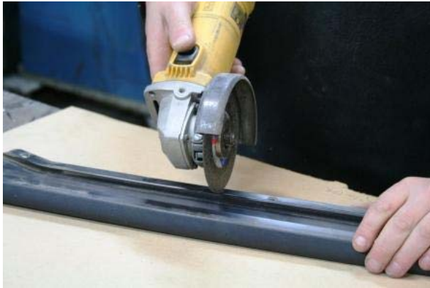
3.39 Grind the black strip along the marks made in step 3.37
