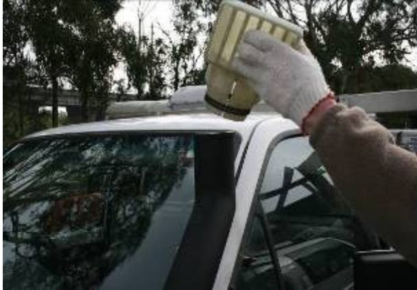
4.1 Remove the Air Ram SP063
