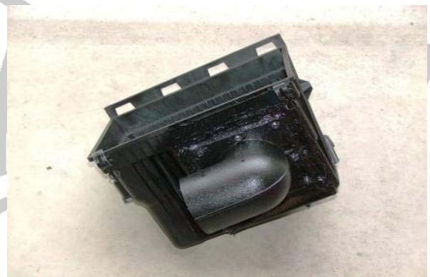
3.19 Smooth out the excess mastic both outside the air box...
