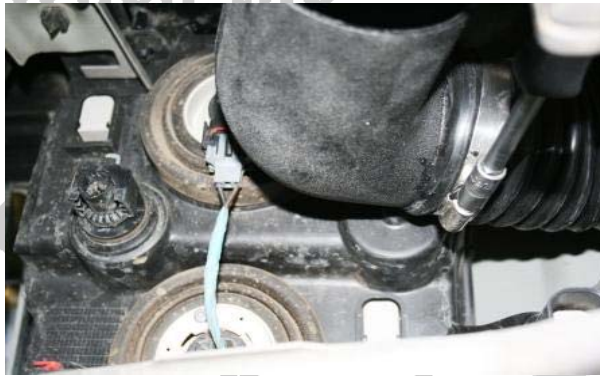
3.65 Slide a hose clamp SP019 on the TPR hose
