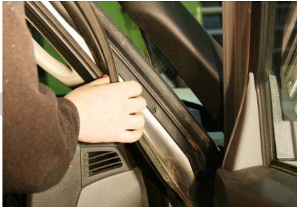
3.35 Peel off the rubber seal from the A Pillar
