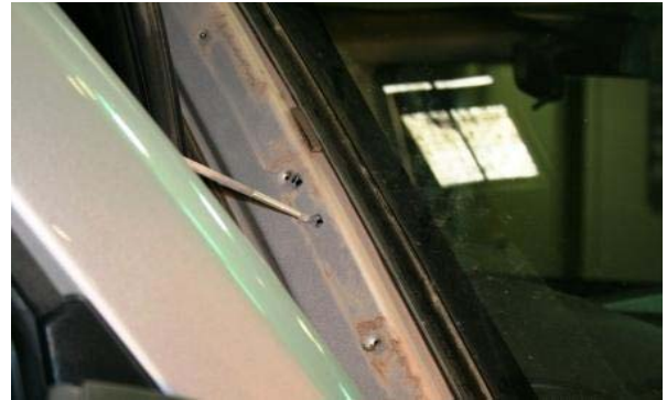
3.48 Paint ALL raw metal surfaces with Zinc rich primer (6 snorkel fixing holes, 1 air intake hole, 2 "A" pillar holes)
