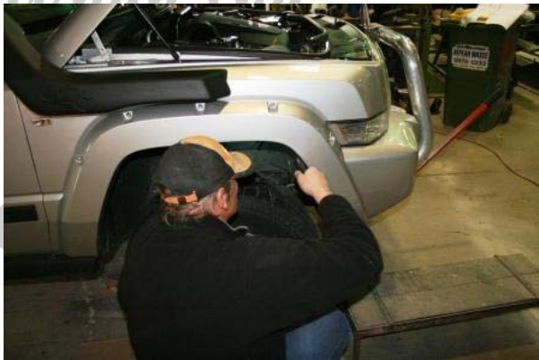
3.75 Refit the splash panel using the plastic rivets previously purchased
