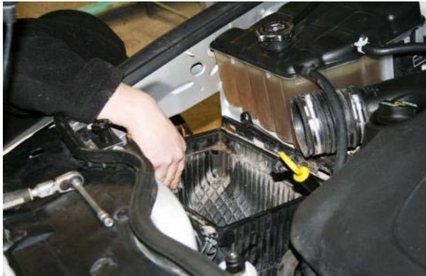
3.72 Secure the air box base in the engine bay
