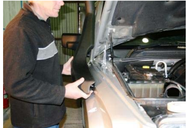
3.34 Fit temporarily the snorkel SP168 to allow the marking of the "A" pillar bracket
